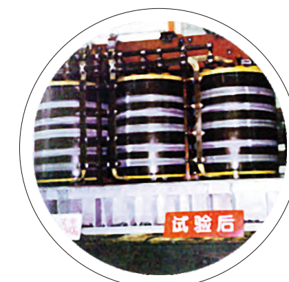
The 110kv Transformer Passed Short Circuit Withstand Test
