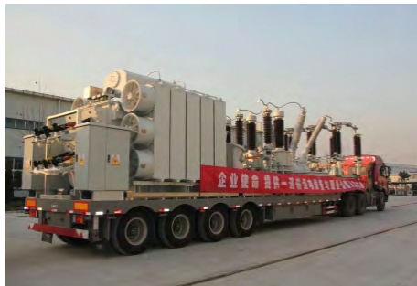
66KV Mobile substation
